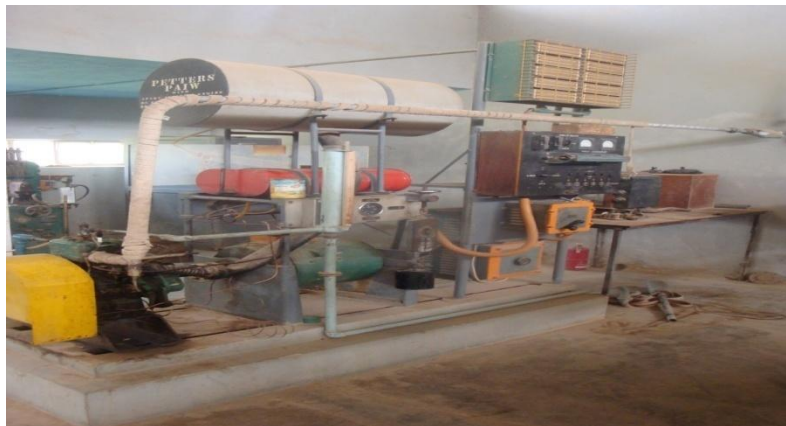
Figure 1: A pictorial view of the Peters PIAW S.I engine used in this study.
